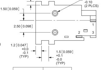
**SCHEMATIC** Model PJ-041H Center Pin Ø1.65 mm
